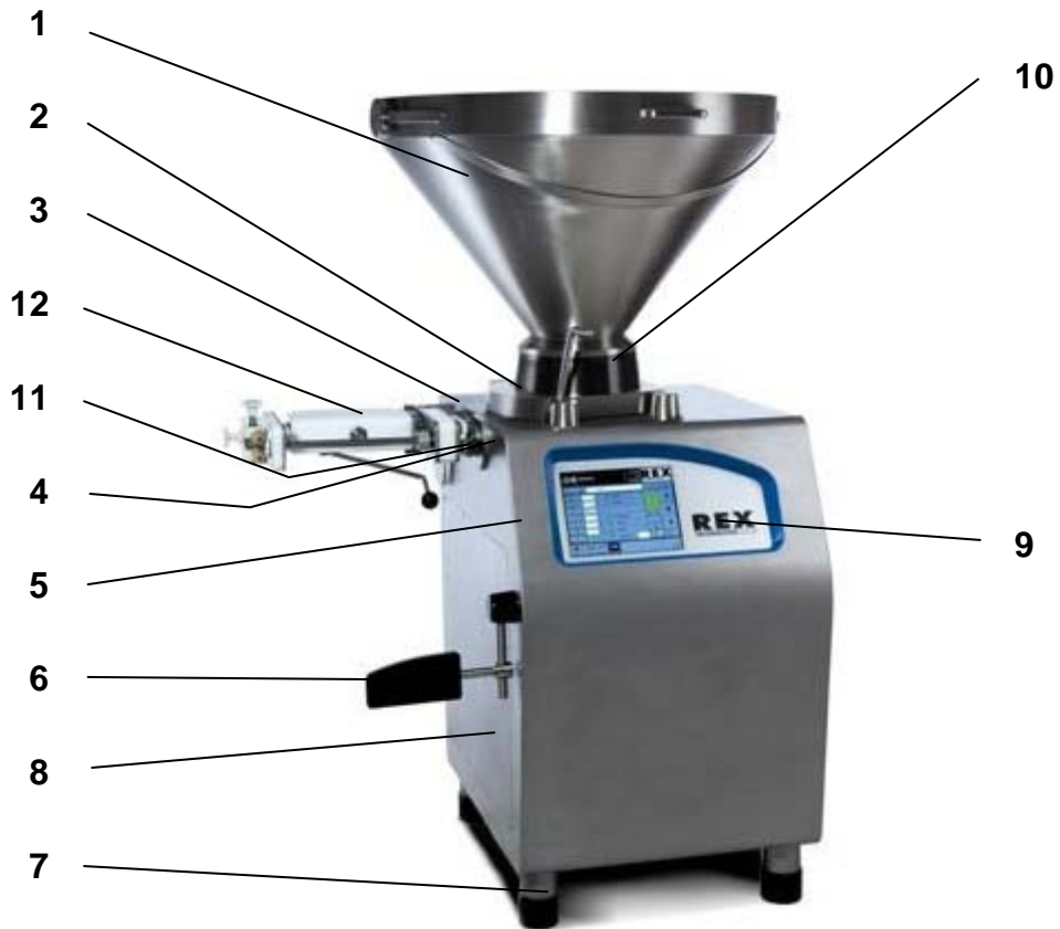
Illustration 3: function elements and their arrangement on the vacuum filling machine
